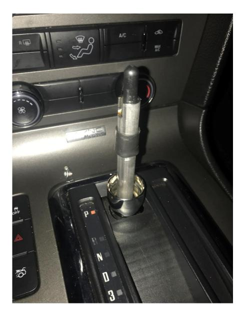
Step 5- Once the chrome piece is slid in place install the tiny screws that hold the new knob in place into the shift knob itself. The little black rubber piece is optional. I preferred to use it to help hold the knob in place better.
