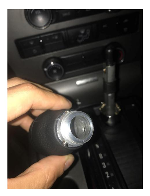
Step 6- Once the screws are in place slide the new knob onto the shift pole at your desired height and tighten the screw to hold it on place. Once at desired height slide the chrome piece up and screw it onto the bottom of the shift knob and the install is complete. Enjoy your new shift knob!
