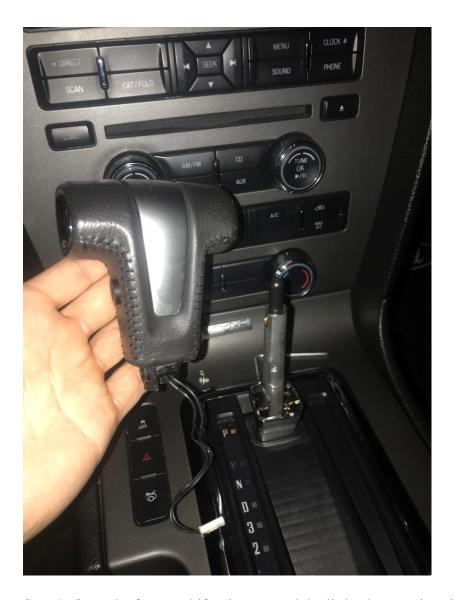
Step 4- Once the factory shifter is removed the little chrome piece just slides off the rest of it. Unscrew the chrome piece of the new knob and slide it down to the bottom on place of the old chrome piece.
