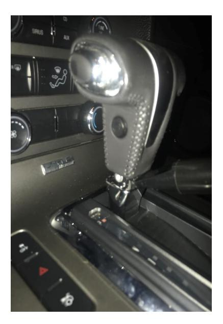
Step 3- Once the screws are exposed remove them. There is one on each side of the shifter. Once removed the shofter should slide right off. Remember if your vehicle has hill assist you will be disconnecting that feature. Be careful when lifting off the factory shifter because the hill assist will still be connected. I pulled slowly but firmly and it popped right off. Notice the white connecter for the assist button.
