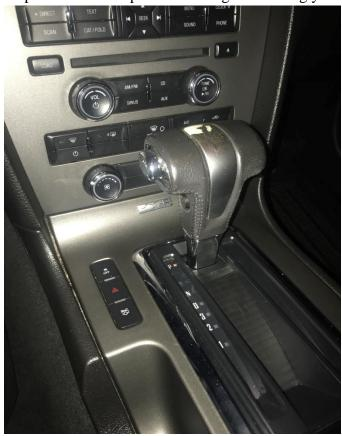
Step 2- To begin removing the factory shifter you have to separate the little chrome piece from the rest of the shifter. In order to do that you will need to pry it apart from the shifter by using your flat head or item of your choice and apply downward pressure. This will expose the torx screws holiding the shifter in place.
