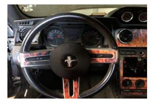
1. Disconnect the battery (ground) and wait 5 to 10 minutes to insure the power has drained out of the system. If you want you can also pull the airbag fuse from the SJB found on the passenger side kick panel fuse #17 which is 10 amp fuse.
