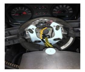
6. Use 24mm socket to remove the main steering wheel bolt.
