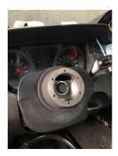
11. Now use the horn mount to attach in between the hub and steering wheel
