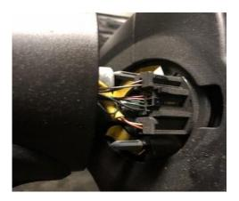
5. Disconnect the cruise control electrical connector, you will see a tab at the top of the connector, use a small flat screw driver to lift up tab and pull out on connector to remove.
