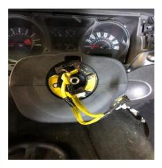
8. Take out four torq bolts with t10x4 torque driver on the clock spring to remove
