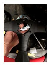
12. Now mount the steering wheel and horn mount to the hub with the supplied torque screws
