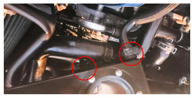
16. After the lower fastener has been attached, bolt in the two (2) smaller (8mm) fasteners into the top of the radiator support beam. Tighten the bolts snug and then snug the lower bolt as well.
