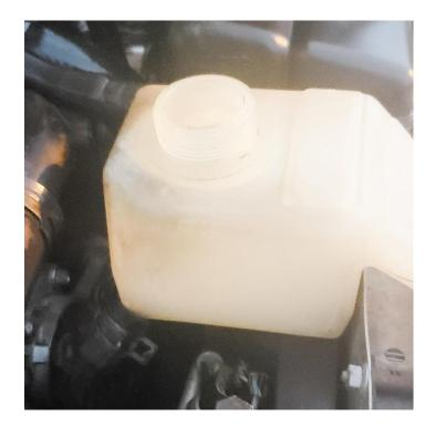
6. Once all the fluid has been removed from the tank and set aside, remove the two (2) fasteners that hold the tank to the radiator support beam using a 8mm socket and ratchet.
