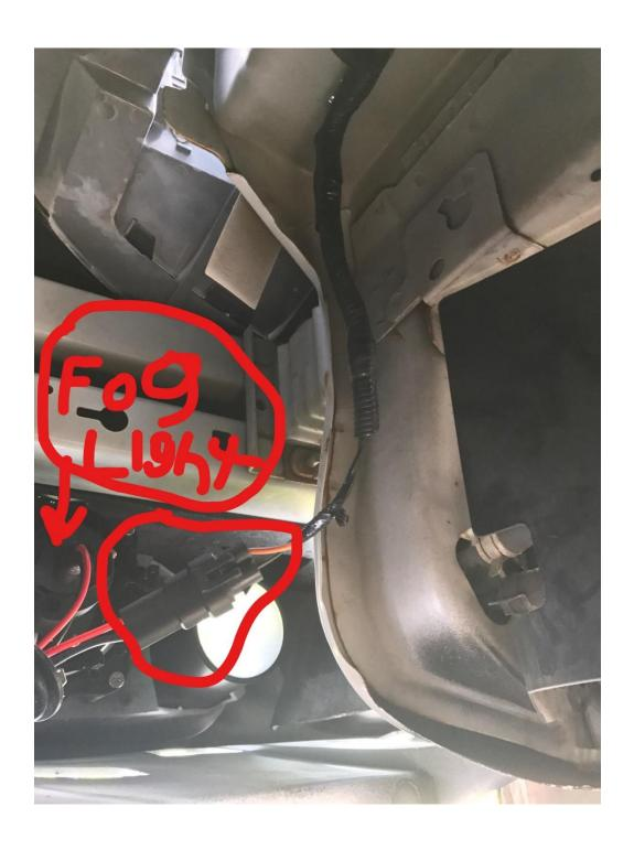
Step 6: Now you just have this last step before removal. Unbolt the 4 11mm Bumper bolts holding the bumper to the car. There are 2 on each side. They are located where right on the inside of upper fender wells. Refer to pictures. Note mine are covered by HID Ballast Stock will not be.
