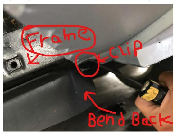
Step 4: Now unscrew fender well retaining screw again there are 2. Note this will allow you to peel back plastic fender well to get at the Bumper bolts and the fog light plugs. Location in picture.
