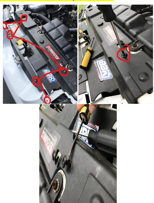
Step 3: Now under the car remove clips connecting the bumper to the frame to yet another trim piece by prying them with a flat head. Note be careful removing these clips as they are well known to break or have an extra set handy there are 2.
