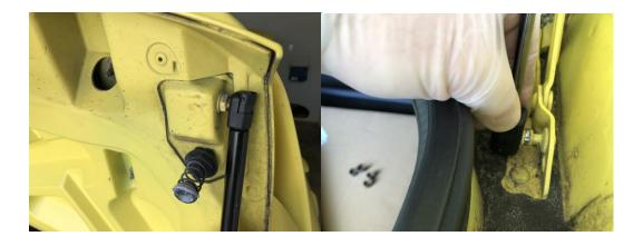
6. Both OPR Trunk Struts Installed and the trunk lid now pops open and stays open!
