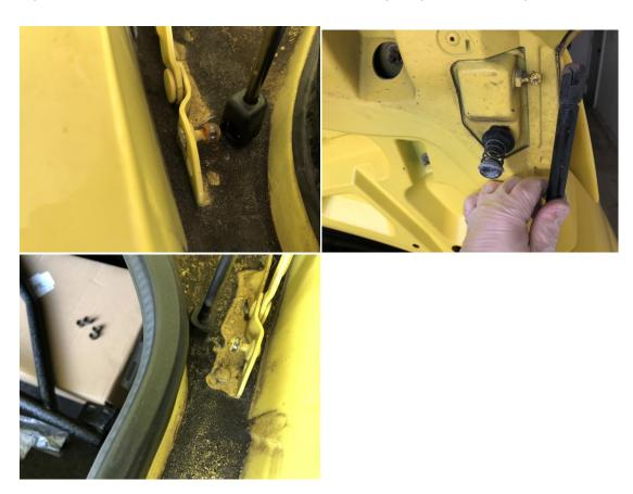
5. Put on new strut and lock clips, repeat for other side
