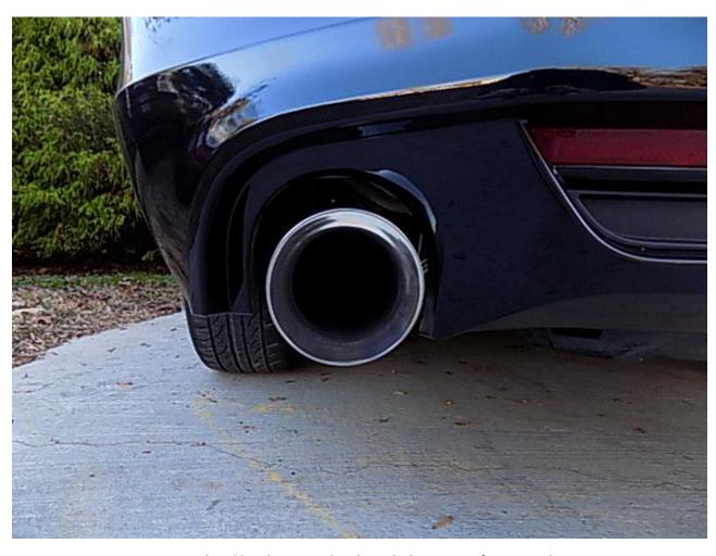
• Step 9: Once centered and level Torque the clamp bolt to 32-35 foot pounds
