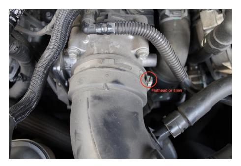
6) This should allow you to remove the entire stock intake assembly as a whole. Don't forget to remove the MAF sensor and keep it safe as you will need it on the new intake.
