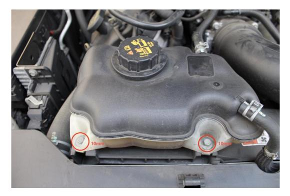
9) Using the relocation bracket and the provided hardware (M4 hex bolt head, washers, and 11mm nut), move the coolant tank over.
