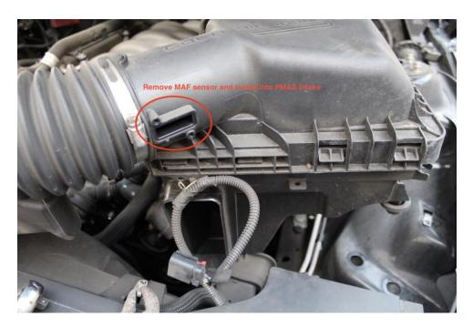
7) Remove the stock airbox plastic piece that is hidden near the brake unit.
