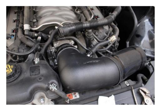
12) Reconnect the 2 hoses disconnected earlier. 1 of them is the sound tube. This can be deleted by using the provided firewall plug. Or you can connect this to the intake to retain the sound tube.
