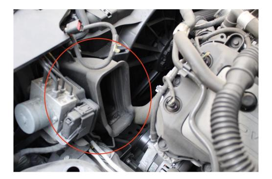
8) Because of the large PMAS intake size, the stock coolant overflow reservoir needs to be moved over using the included PMAS bracket.
