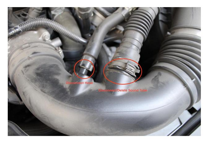
The sound tube can be deleted using the cap that comes with the PMAS intake. (Optional)
