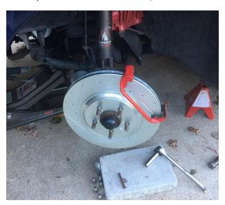
Step 8: Remove the old front brake pad from the caliper, you may need the large flat-head for this. Using your c-clamp, tighten the clamp onto the old back brake pad to slowly push the caliper piston back into the caliper. Once you have fully compressed the piston, you can remove the other old brake pad.
