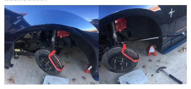
Step 6: With the caliper bracket removed, the rotors should slide right off. If there is a lot of rust, some hits with your hammer will persuade the rotors to come off of the hub.
