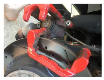
Step 5: With the caliper and pads out of the way, it is now time to remove the two 15mm bolts holding the caliper bracket to the car. These bolts can be very tight, so use a shorter breaker bar and be sure not to round them.
