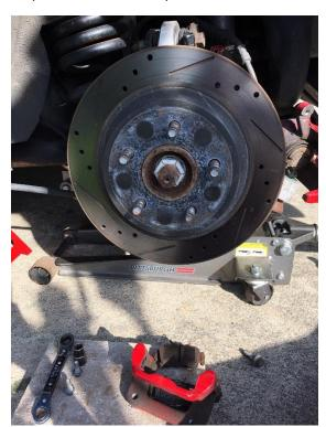
Step 7: You should be able to slide the rotor off now. If the rotor is seized to the hub, use a rubber mallet and hit the top and bottom to knock it loose.
