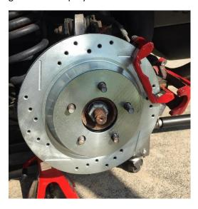
Step 10: Pull the slide pins out of the back on the caliper bracket. These pins should be moving freely. If not, clean them off and apply some grease to the pins and re-insert them.
