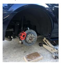
Step 2: With the wheel off, use your 12mm ratcheting wrench or crescent wrench to loosen the two bolts holding the caliper to the bracket. There is limited room, so a regular a ratchet/socket combo is unlikely to fit.
