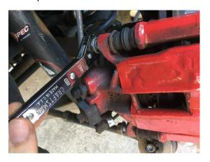
Step 3: Lift the caliper off of the pads, you may need a flathead to assist if the caliper is too tightly fitting. Secure the caliper somewhere so that there is limited stress on the brake line.
