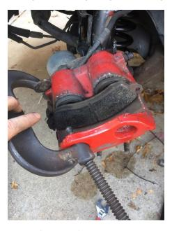
Step 7: (Optional) lightly spread some caliper grease on the back of the brake pads to reduce any metal-to-metal contact noises and squeaks.
