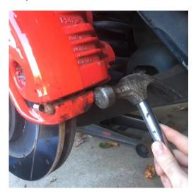
Step 5: Tilt your caliper up into the air until it is completely separated from the caliper bracket.
