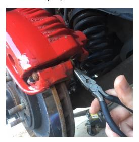
Step 4: With the clip removed, lightly tap the back of the pin with your hammer until you are able to pull the pin out.
