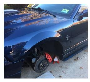
Step 3: Begin by removing the C-clip that holds the caliper bolt in place. Some needle nose pliers will come in handy to pull it off.
