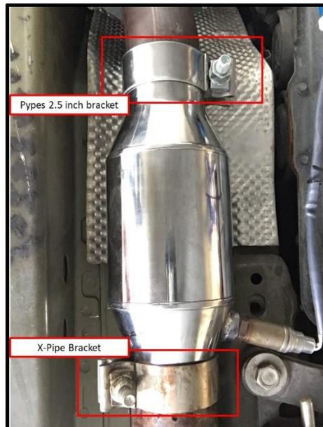
Figure M: Pypes 2.5 inch bracket and X-Pipe Bracket with O2 Sensor
