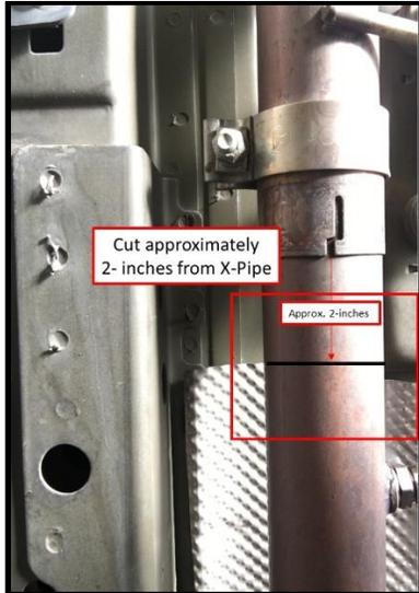
Figure I: Mid-Pipe Cutting Location
