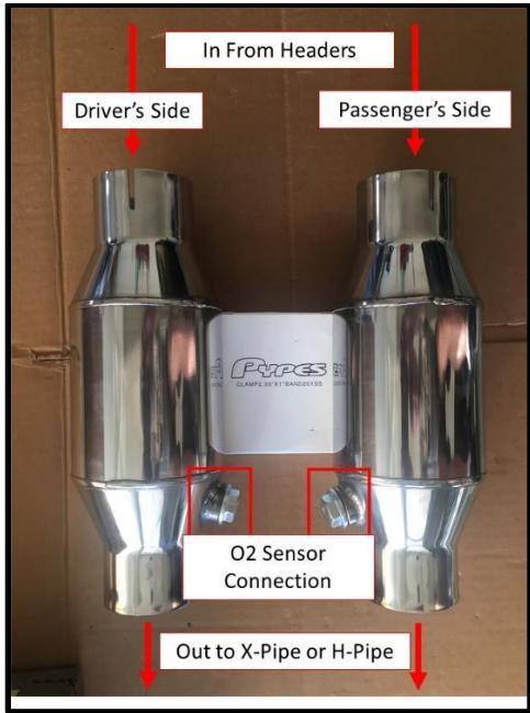
Figure B: Catalytic Converter Orientation
