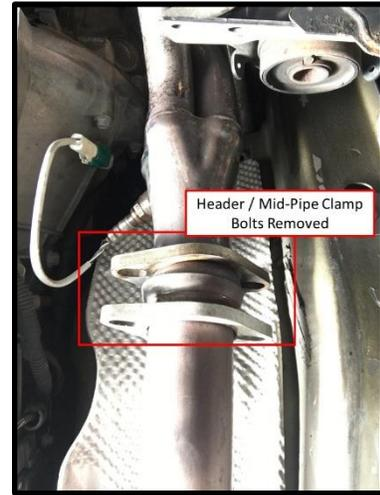
Figure F: Bolts Removed
