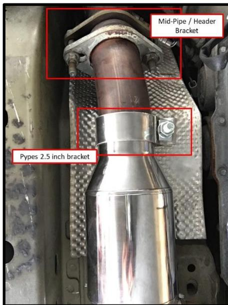
Figure L: Mid-Pipe Header Bracket
