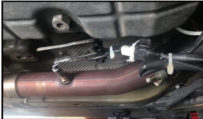
Figure A: Mid-pipe without Pypes High Flow Metallic Catalytic Converter
