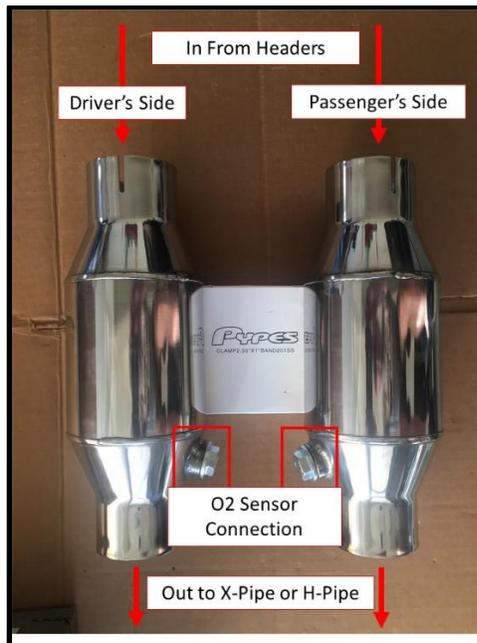
Figure B: Catalytic Converter Orientation
