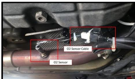
Figure B – O2 Sensor cable and O2 Sensor
