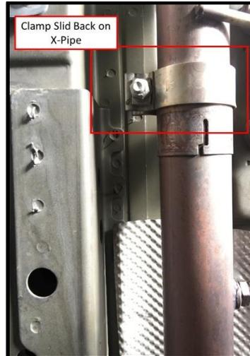
Figure H: Clamp Slid Back Onto X-Pipe
