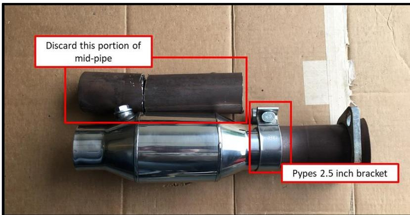
Figure K: Mid-Pipe Inserted into Catalytic Converter
