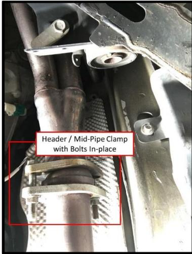
Figure D: Bolts In-Place
