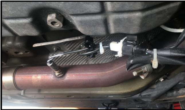
Figure A: Mid-pipe without Pypes High Flow Metallic Catalytic Converter
