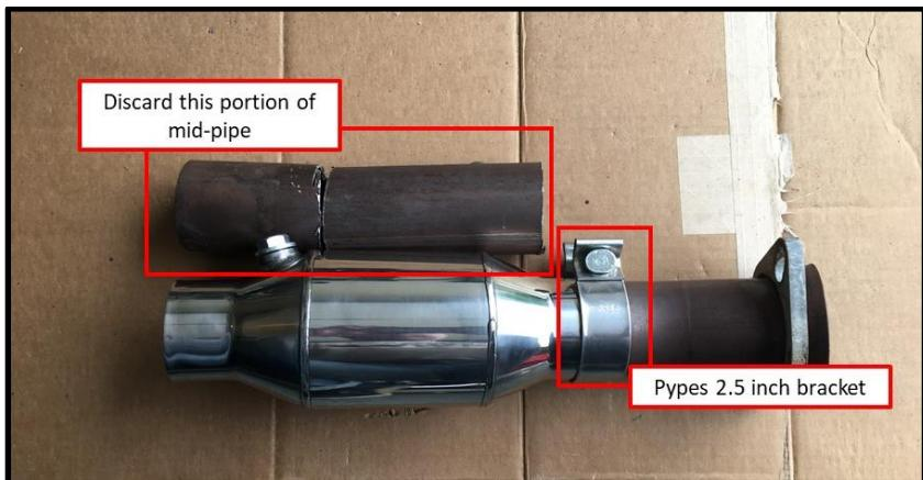
Figure K: Mid-Pipe Inserted into Catalytic Converter
