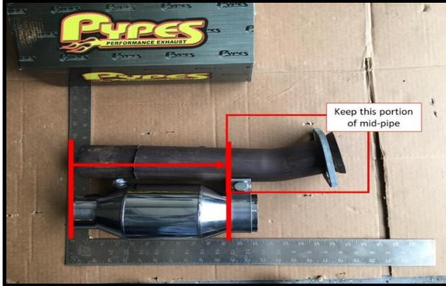
Figure J: Mid-Pipe and Catalytic Converter Alignment for Cutting
