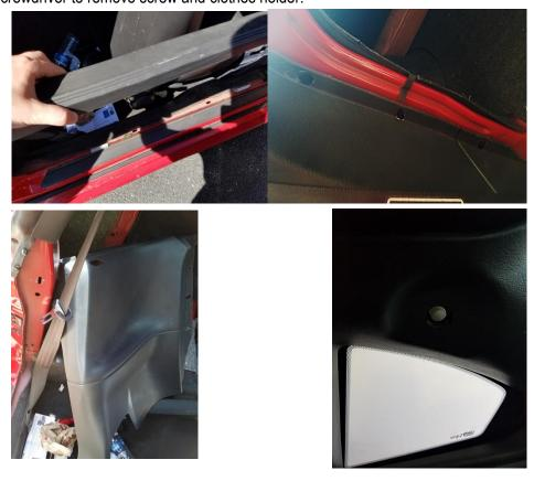
13. Once done, you can now remove the second bolt for the seat belt which is behind the arm rest interior panel.
