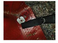
11. Then use a T-50 torx with a 3/8" drive to start the removal process of seat belts. You start by removing bottom of seat belt bolt. But make sure and put the bolt back to keep water out of cabin of car. I put the bolt back as you can see in the second picture.
