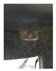
6. Then use 3/8" drive with 10mm socket to remove 2 bolts under head cushion. These bolts will be last thing holding the seat bracket to the car.
