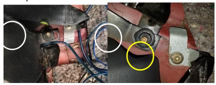
(The dark nuts are the ones needing to be removed (ones with white circle), the goldish bolts are the T-50 torx bit you will use later to remove your seat belts.(ones with yellow circle)
