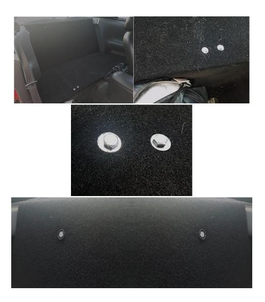
\*(These pictures are in order, the final seat delete kit, than the bottom bolts and washers from left to right side, than the back of the seat delete from left to right with given hardware.)
