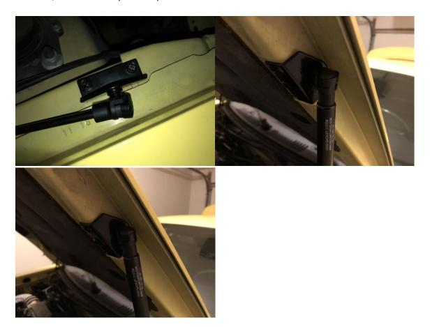
19. Once both sides are attached you can raise and lower your hood with ease and no unsightly prop rod, you can remove the prop rod with a 5/16" socket and ratchet.
