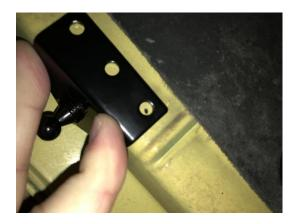
5. Use your center punch and hammer to indent the permanent marker to help guide the drill bit and keep it from wandering. Drill out the hole using your 3/16" drill bit, however be very careful as to not go too far through as you may damage the hood.
