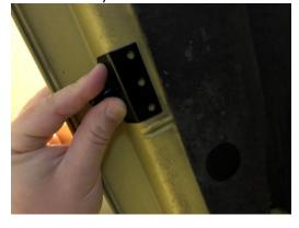
4. Holding the angled bracket flat against the hood. Using your permanent marker place a dot in the center of bottom hole.
