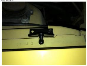
15. Once that screw is tighten down, make sure your bracket is parallel with the fender, mark the other hole, center punch the hole, drill it out using the 5/32" drill bit and attach the other side of the bracket with the self taping sheet metal screw.
