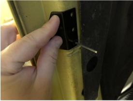
7. Once you have the bracket and rivet in place, slid your rivet gun onto the stem and while applying downward pressure firmly squeeze the rivet gun until the rivet pops. Now your bracket should be held in place.
