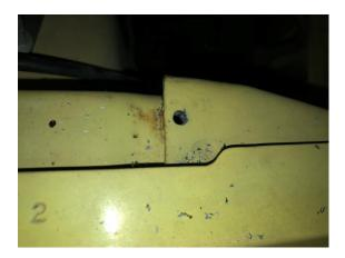
14. Place your bracket over the hole, using the included self taping sheet metal screws, place one screw into the hole and tighten down, you can use a 5/16" socket and ratchet but I would recommend using the drill with a 5/16" nut driver attached or an impact driver with a 5/16" socket.
