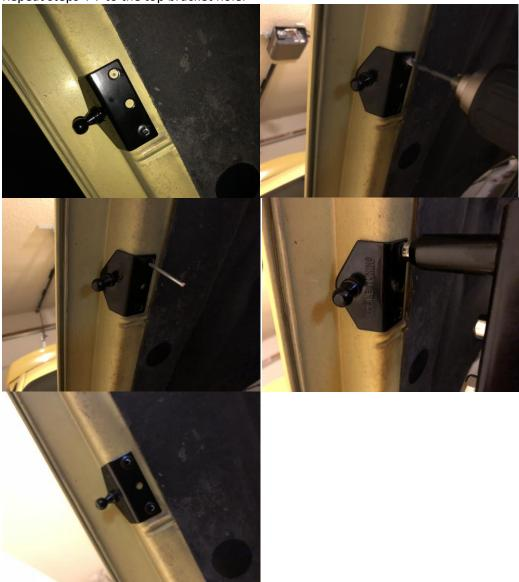
9. Repeat steps 4-7 for the center bracket hole, using the longer rivet.
