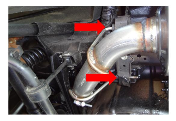
9. Insert the rear most metal rod into the rear most rubber grommet.
