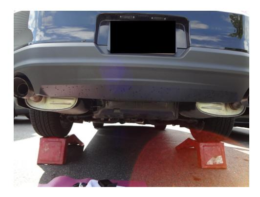
2. Loosen the bolt on the clamp that is holding the stock muffler to the over axel pipe. (Do one side at a time).
