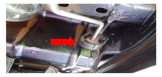
10. The pipe leading to the over axel pipe should be fairly lined up. The over axel pipe will go around the outside of the ROUSH muffler. Slide the clamp so that half is on the muffler and half is on the over axel pip. Make sure that the muffler is inserted fully into the over axel pipe and then tighten it down until the two metal ends are touching.
