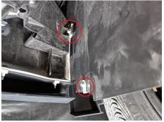
12. Install 2 of the provided 8mm black bolts to hold the canards to the fender liner and bumper.
