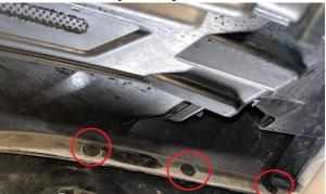
5. Remove (8) 7mm screws securing factory chin spoiler to the bumper. Remove the chin spoiler completely from the bumper.
