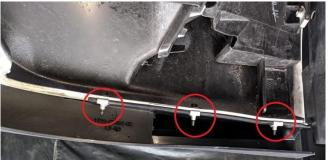
14. From underneath of the vehicle, install the 2 provided 7mm self-tapping screws and drill one into the bottom of each canard to hold the chin spoiler and canards together.
