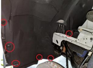
3. Underneath the vehicle, remove (17) 7mm bolts and 2 push pins securing the belly pan to the subframe.
