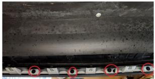
6. Install the provided J-clips onto all of the holes on the Roush chin spoiler, threads towards the front of the vehicle.
