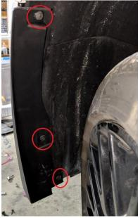
13. Install the new Roush chin spoiler by aligning the nipples on the spoiler and then securing it to the bumper with the provided 7mm silver screws.
