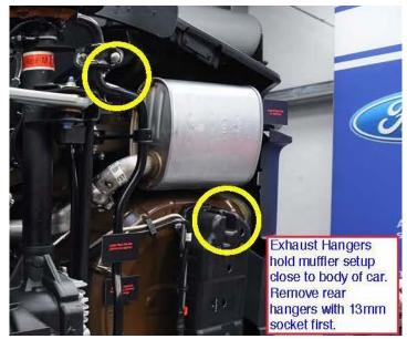
sticks through the hanger bolted to the vehicle. The hanger bolted to the vehicle is what is to be removed. The bolts and hangers are all needed for reinstall so do not loose these.)
