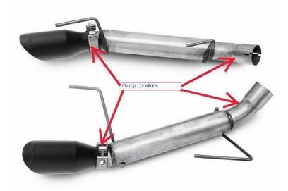
7. Start by getting under the car with the new pipe. Install the hanger closest to the end that will connect to the mid-pipe. (The metal hanger on the pipe will go through the same hole the stock muffler went through) After inserting that hanger, install new pipe over the mid-pipe. (Make sure that your exhaust clamp is still on your pipe. Do not concern yourself with tightening this yet. You will need the room to work.)
