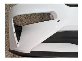
16. Flip the bumper face down on a soft surface and grab the third template and align it under the fog light cutout close to the lower grille and tape into place.
