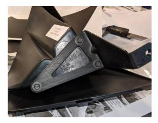
21. Stick the supplied double sided 3M tape to the back of the Roush pocket along the front-most part.
