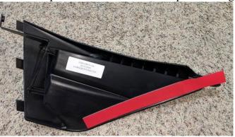
22. Remove the other side of the tape and prepare to install onto the bumper. Line up the 3 tabs with the 3 holes drilled out. The stud will line up with the large hole drilled.
