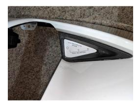
12. Drill the mark first with the 1/8" drill bit followed by the 1/4" drill bit.
