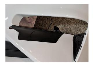
20. Install the metal bracket onto the pocket using the (6) supplied 7mm screws.
