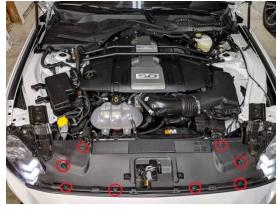
3. Remove (6) 8mm bolts and (2) 5.5mm bolts that secure the bumper to the core support.
