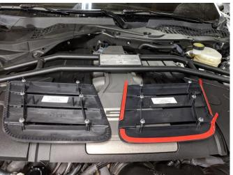
11. Pull off the other side of the tape and install the extractor to the hood applying even pressure.
