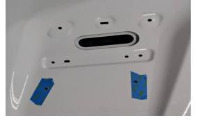
6. From the underside of the hood, drill the outermost holes using the 1" hole saw only going through the skeleton of the hood. DO NOT go through to the skin of the hood.
