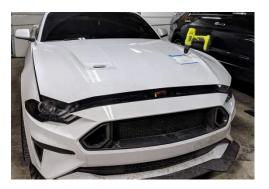
5. Using a center punch, mark where the holes will need to be drilled towards the rear of the hood. Start by drilling a 1/8" hole. Drill the same holes with the 7/32" bit next. Be sure to go completely through both layers (skin and skeleton) of the hood.
