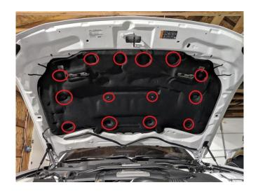
2. Remove (4) 8mm sockets securing the factory vent backing and pry off. They are held on using adhesive tape.
