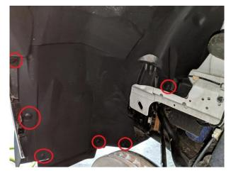
5. Remove the (2) 10mm nuts that hold the bumper to the fender and pull the black bracket (pull straight down). This is secured by a push pin.
