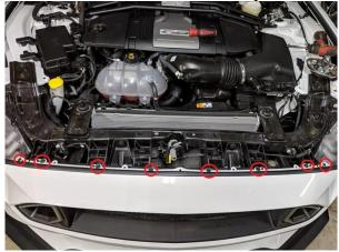
4. Remove the 6 push pins to allow the inner fender liner to be pulled back. Pull this back and tuck out of the way.
