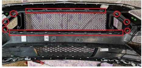
13. Prep the new grille for install by drilling (6) 3/16" holes in the marked spaces. (innermost part of the
