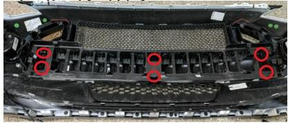
12. Remove factory grille by gently prying the tabs. Using a wide flat head screwdriver makes this step easier.
