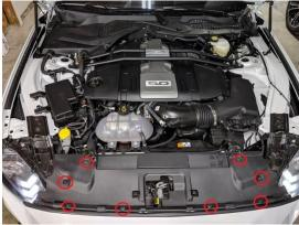
3. Remove (6) 8mm bolts and (2) 5.5mm bolts that secure the bumper to the core support.
