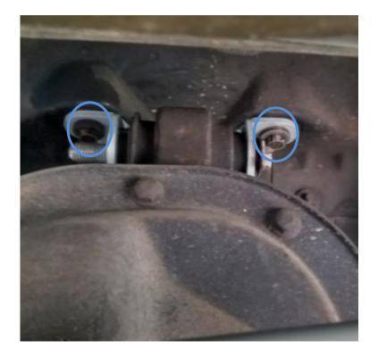
11. Tighten the upper control mount bolt located underneath the back seat using 24 mm socket/wrench and stock bolt.
