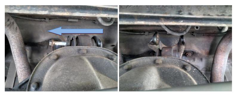
5. Unscrew the upper control mount screw using 21 mm socket/wrench and extension.
