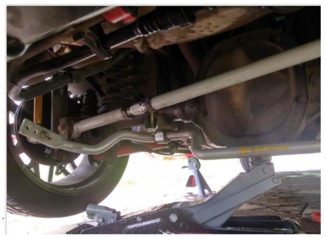
4. Remove the differential bushing screw, in case of problems use a hammer and small punch. Avoid hitting the thread of the screw.
