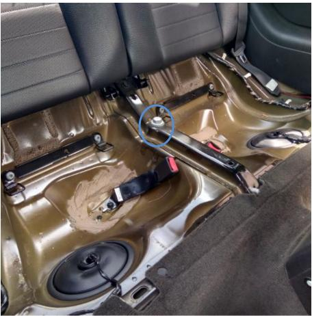
12. Tighten the upper control arm to differential bushing using 18 mm socket/wrench and stock bolt and nut.
