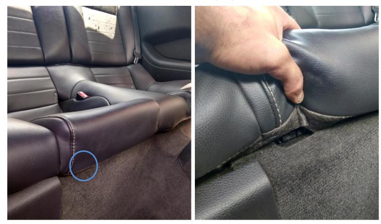
7. Unscrew the upper control arm mount screw number 3 located underneath the back seat using 24 mm socket/wrench.
