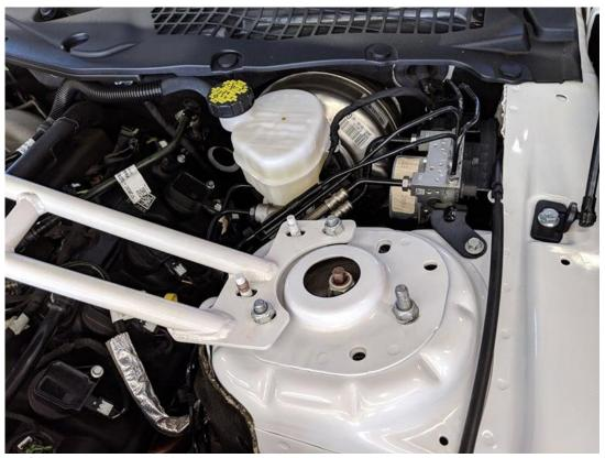
• Safely compress the spring and remove the 21mm nut that secures the strut to the top hat
