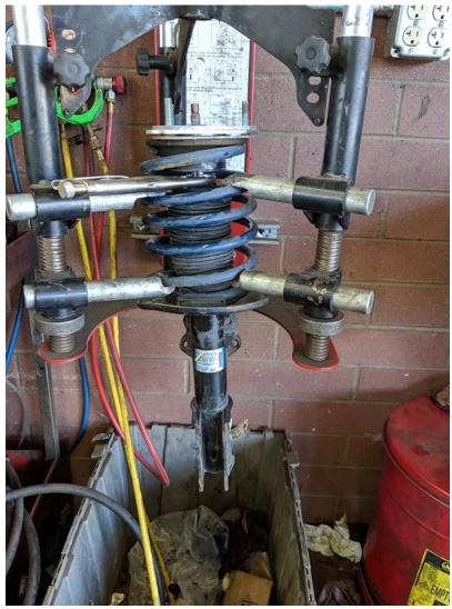
Once they are separated, remove the bump stop/ dust boot along with the bottom rubber spring seat
