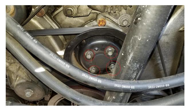
**6.** Now that the four pulley bolts are broken loose, remove the serpentine belt. This is a great time to replace the belt if it is old, cracked, or damaged. Insert a 1/4" socket into the belt tensioner and rotate it clockwise to loosen the belt and slide it off. A breaker bar will make the job much easier. Then finish unscrewing the loosened pulley bolts and remove the pulley.
