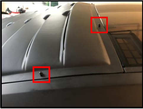
Figure I: Nut and Wash Reattached to Attachment Bracket
