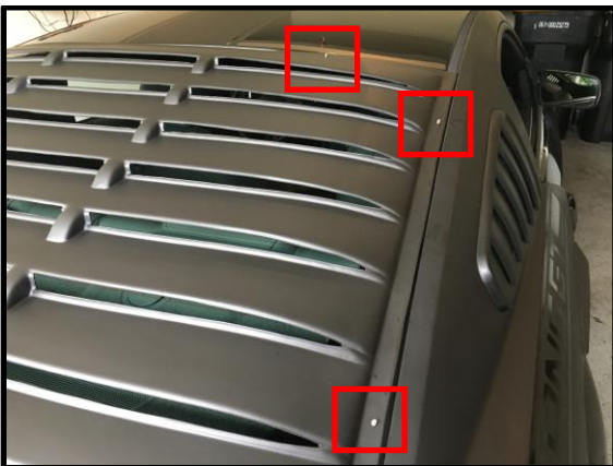
Figure H: SpeedForm ABS Rear Window Louvers Attached with Attachment Bracket Pegs through (3) Holes
