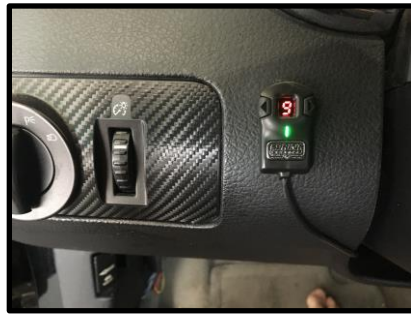
Figure E: Acceleration Mode Settings (Off, Sport, Race)
