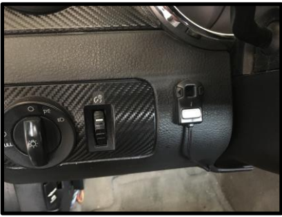
Figure E: Acceleration Mode Settings (Off, Sport, Race)
