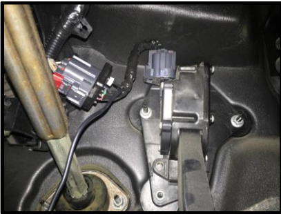
Figure D: Sprint Booster Connected to Pedal and Harness
