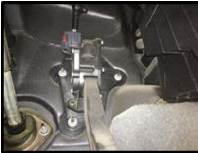
Figure C: Pedal Harness Connector
