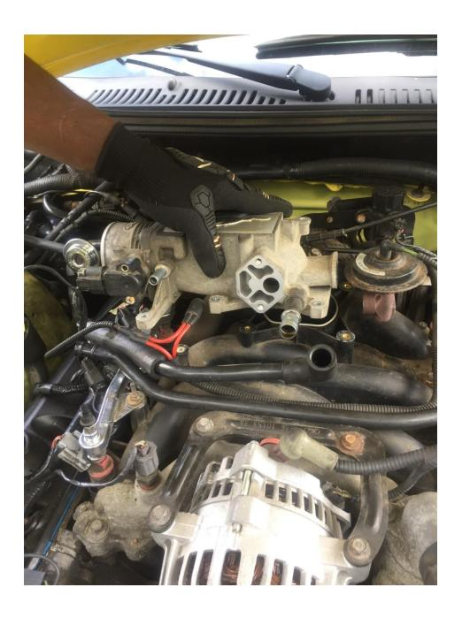
6. Use a 10mm deep well socket and extender with ratchet to remove the two bolts securing the EGR Valve.
