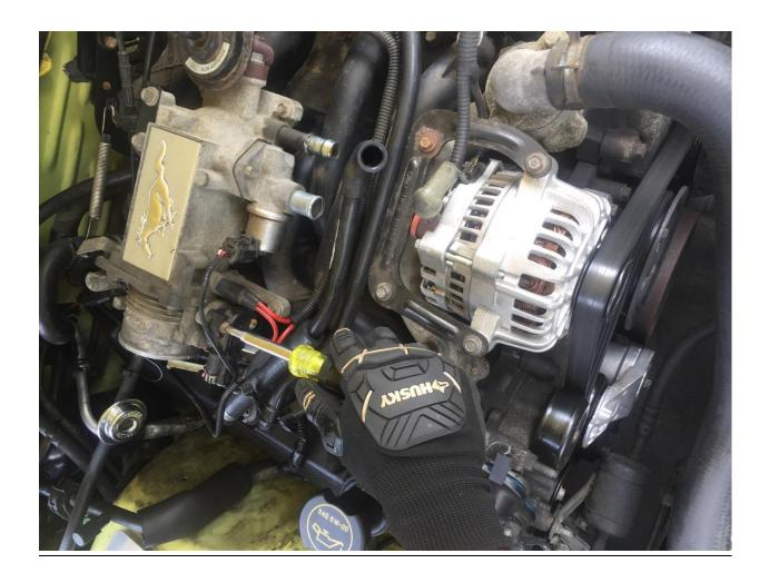
Remove the two 8mm bolts to detach the Idle Air Control Sensor; be careful if you wish to reuse your gasket, although I used the new gasket provided in the SR Performance kit.
