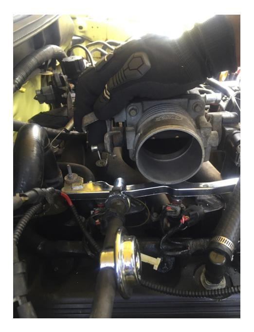
8. At this point, all wires and tubes should no longer be connected anywhere along the four sides of the throttle body. Now, use an 8mm socket to remove all (5) bolts along the edges of the throttle body and lift it from the car. If you will not immediately be installing the new throttle body, take a clean shop towel and cover the manifold opening to keep clear of debris.
