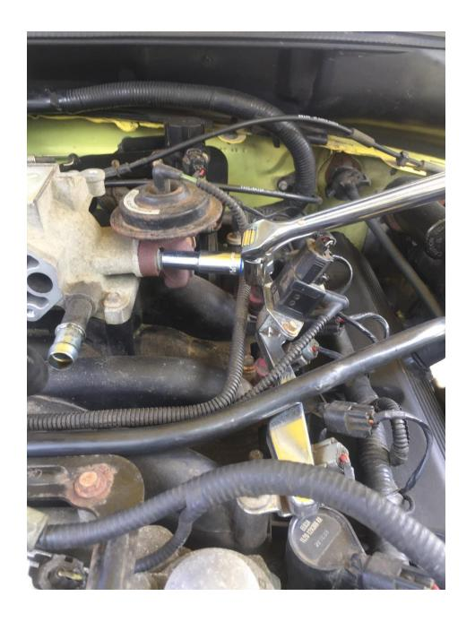
7. Next, move to the back of the throttle body to the butterfly valve and remove the two 10mm bolts securing it. Next, pull down slightly on the valve to open the throttle in order to provide enough slack to pull the throttle cable out of the cam guide. Next, pull out the spring.
