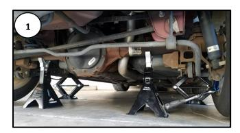
2. Use the 15mm Deep socket to remove the bolts from each bushing mounting bracket (4 total bolts). Remove the locking nut/washer assemblies as these will not be reused. Pull bushing mounts away from mounting holes.
