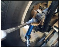
8. Place the vehicle on the ground or wheel ramps under its own weight. Completely tighten all connections made on rear sway bar. Recommended 40 lb-ft for sway bar bushing brackets; end links should be tightened until rubber bushing is contacted on both sides by metal chassis and slightly compressed.
