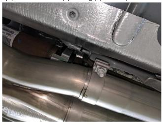
7. Install driver and passenger side tailpipes using (2) 3" clamps, one for each side.
