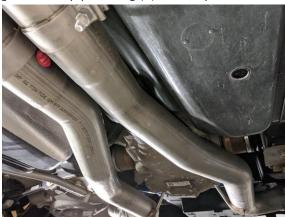
8. Install driver and passenger side mufflers into the rear hangers and onto the tailpipes using (2) 3" clamps, one for each side.
