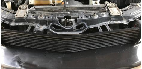
Step 2: Screw in the studs as shown below
