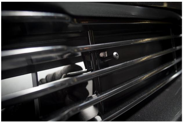
Slide the hardware in from the back of the bumper until the L part's hole lines up with the screw hole in the bumper. Ensure that the J part of the hardware hooks onto your lower grille. At that point, you can screw it in, making sure to screw it only tight enough to secure the grille in place and not damage your existing lower grille. Repeat for the other side.
