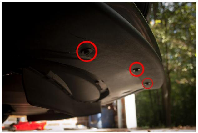
6. Begin removing the 7mm bolts securing the bumper to the close out panel.
