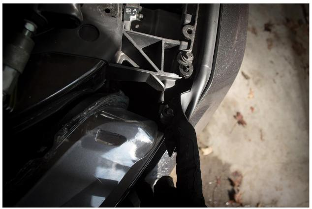
3. Remove the two 7/32" bolts hidden beneath the bumper-hood seal on either side of the bumper.
