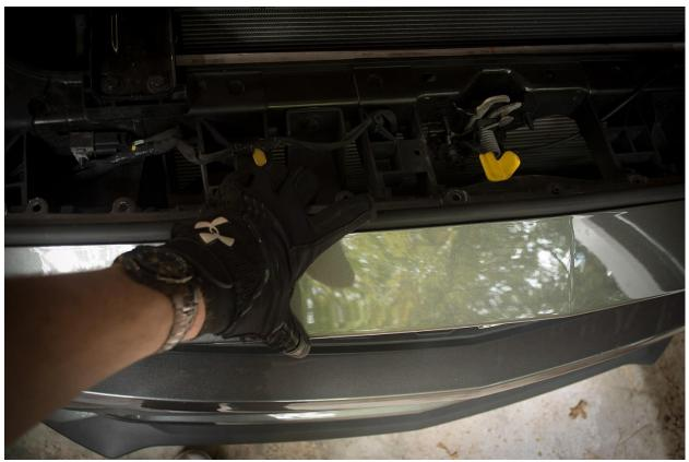
8. Once all the push pins and bolts are unsecured, you can lift the top of the bumper off of the car, unsecuring it.
