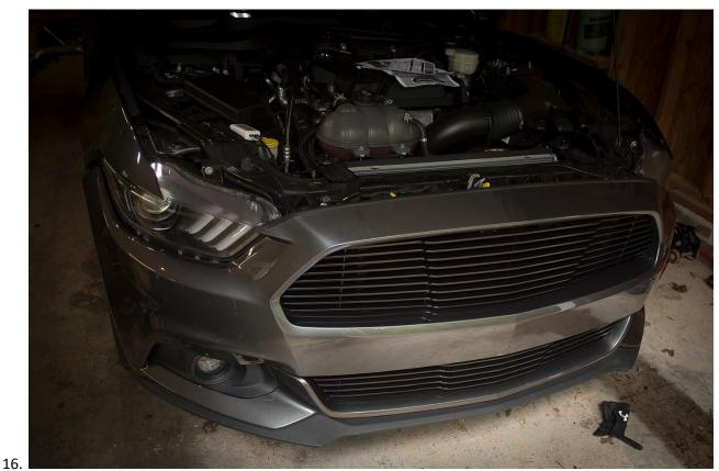
At this point, you can replace the bumper, reconnect the turn signals, parking lights, and fog lights, begin re-securing the bolts by reversing the steps taken to remove the bumper, reinstall the radiator cover, and wiggle\pull\push on the new upper grille a little to make sure it is secure.
