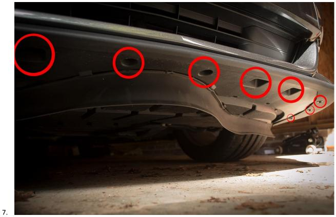
There are some located within the recesses on the bottom of the bumper. In total, you will have to remove twelve screws.
