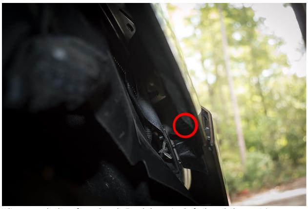
Whatever you do, do not forget about the 7mm bolt securing the fender to the bumper. It is located where the two meet, just behind the splash shield. You will most likely need a 90° drill attachment to remove it.
