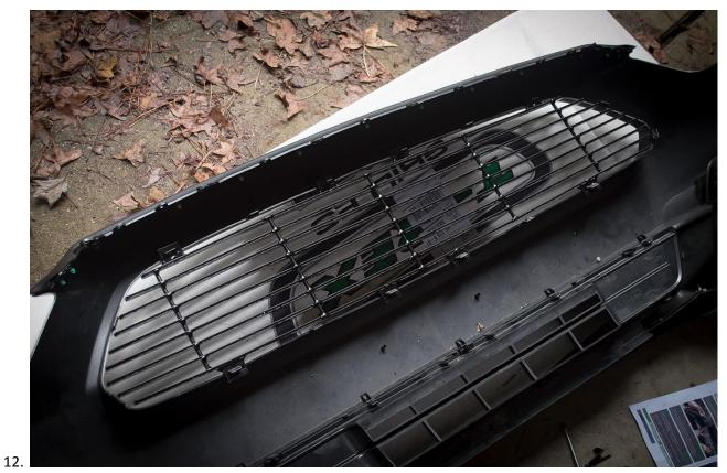
Once the existing grille is removed, you can replace it with your T-REX grille. The clips that held the old grille in place should secure it in place.
