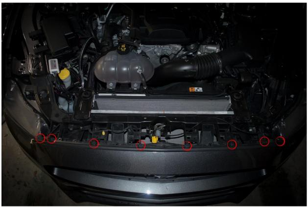
2. Remove the six 8mm bolts securing the bumper to its support, making note of the two 7/32" bolts on either end.
