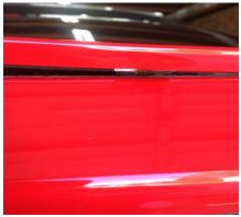
7. Remove excess adhesive left on deck lid using adhesive remover.
