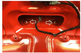
6. Gently pry stock spoiler up to remove. This will take some muscle. Optional: use heat gun to soften adhesive. Also, if able, use razor blade to cut adhesive under stock spoiler to relieve tension. Highly recommend second set of hands.
