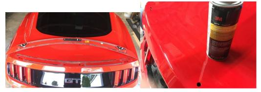
8. Install True Fiber spoiler in same holes using provided hardware.
