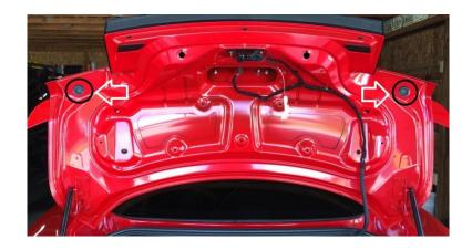
5. Remove (2) 10mm holding center of stock spoiler.
