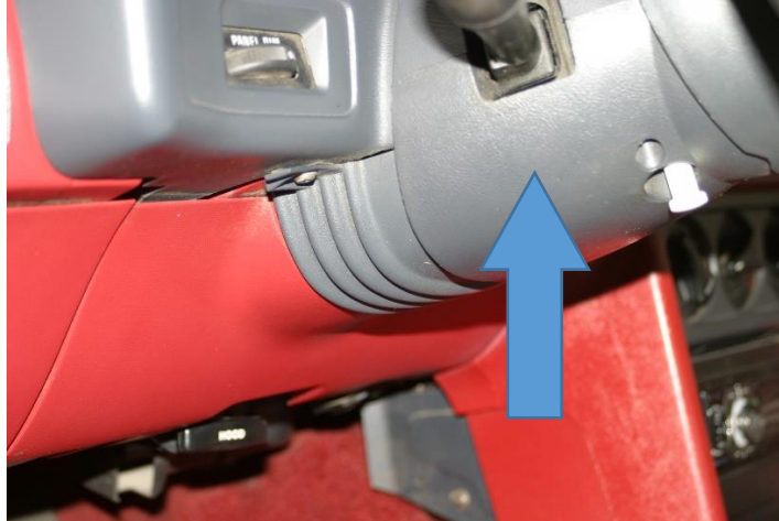
Picture 3: Lower steering column cover as indicated by the blue arrow
