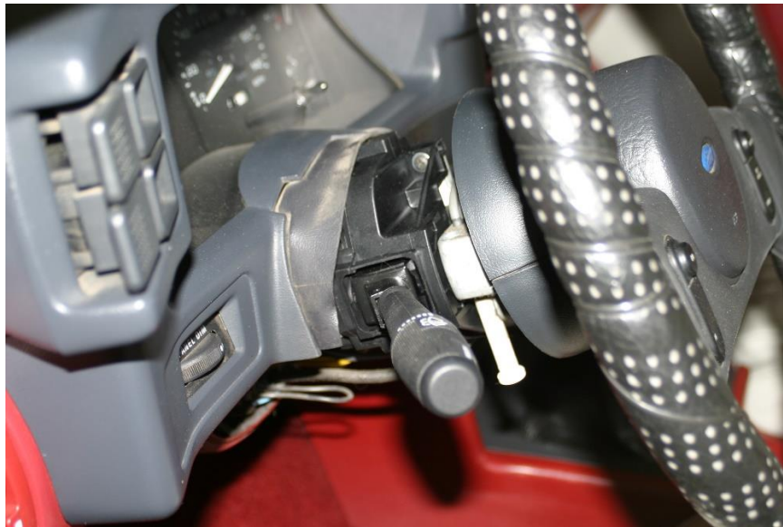
Picture 11: New turn signal installed
