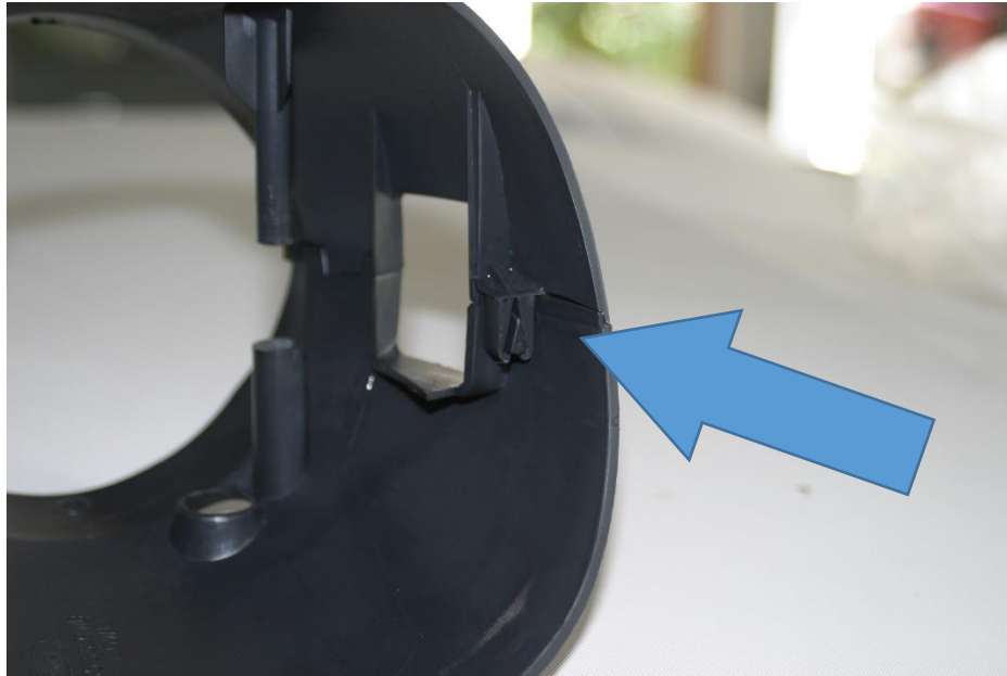
Picture 12: Steering column cover forward snap feature
