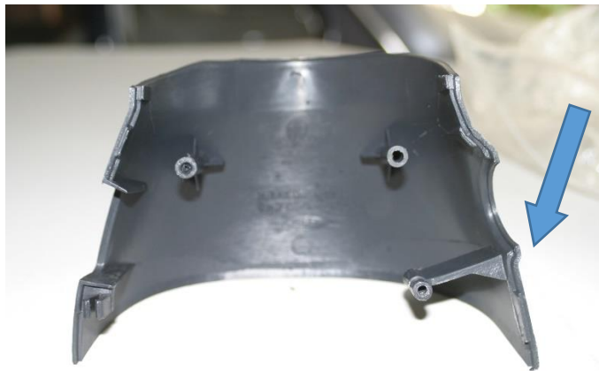
Picture 7: Three steering column screws connect into the top cover.
