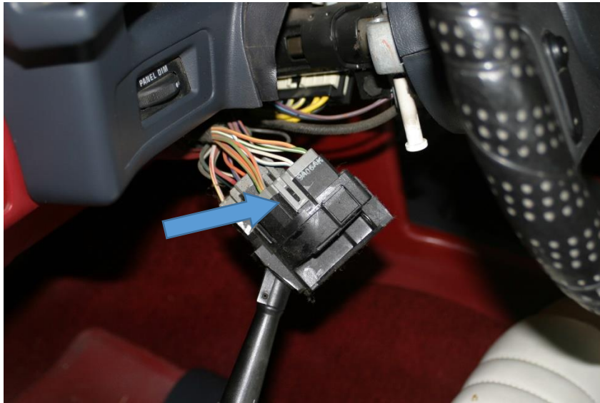
Picture 10: Old turn signal ready for dis-connection
