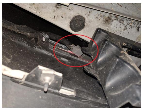
• Now reach towards the front of the car on the marker light and push the tab backwards to release the light.
