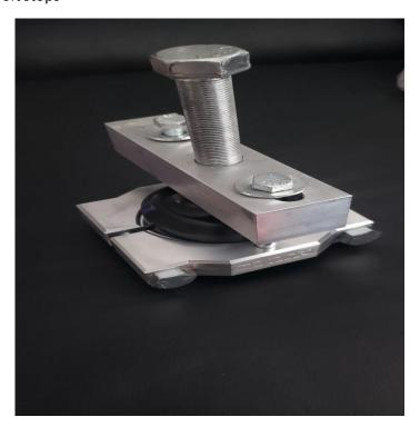
6. Using a Impact gun or Ratchet with a 1 1/8" socket. Tighten **Bolt with Nub** until charger Stock pulley is removed.
