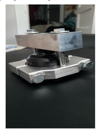
5. Screw in **Bolt with Nub** to the **Removal square** to complete assembly of the **VMP Pulley Tool.**
