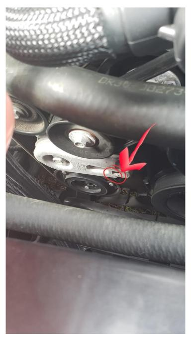
2. Remove black Plastic Cap at then end of the stock supercharger pulley.
