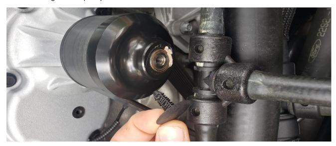
3. Attach **HD Clamp Shell** to OEM supercharger pulley (keep Clamp Shell as far forward on the pulley as possible.)
