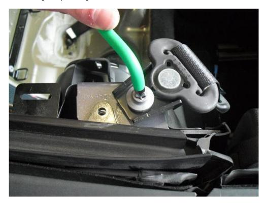
6. Install Styling Bar brackets under factory seat belt guide bolts. **Caution:** Do not use only seat belt guide bolts to secure Styling Bar. Seat belt guide bolts are only used as locaters for the Styling Bar brackets. As show in Step 7, holes must be drilled and provided hardware must be used to properly secure Styling Bar to vehicle.
