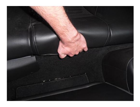
2. Remove the rear upper seat by removing the two 13mm bolts toward the bottom of the seat and pulling up to release the seat from the upper brackets.
