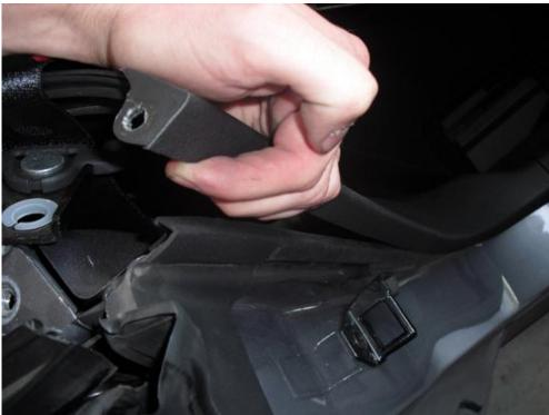
5. Remove seat belt guide by removing 10mm bolt and T50 Allen head bolt.
