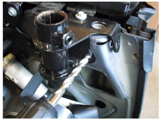
8. Using supplied hardware, secure Styling Bar brackets to body. Make sure to place the nuts on the inside of the body panel, and the Allen head bolts on the outside as shown.
