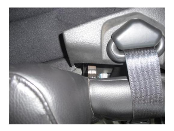
3. Remove upper quarter trim panel by lifting at the shoulder strap opening to disengage retaining clips.
