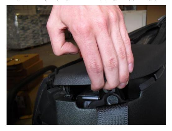
4. Remove lower quarter trim panel by carefully prying retaining clip that holds panel to body, and then pulling panel out towards front of vehicle.
