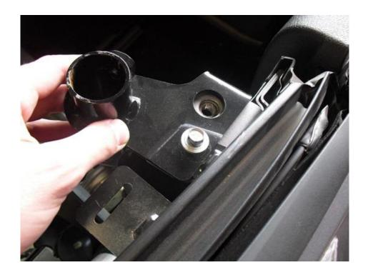
7. Using brackets as guides, drill 1/8" pilot holes through body sheet metal. Follow with 5/16" bit to enlarge holes to proper size.
