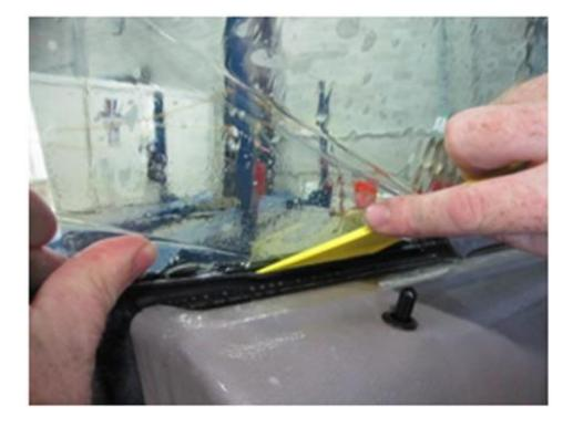
6. Once the tint is fully secured under the rubber trim, use the squeegee to push out any remaining air bubbles. Be sure to use plenty of solution to keep the surface well lubricated so as not to wrinkle the tint.
