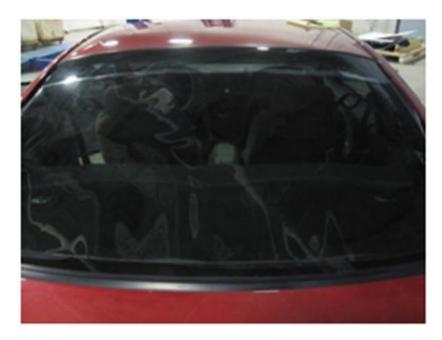
2. Using a heat gun, heat the tint until it begins to slightly wrinkle while pushing it to the edges with the squeegee, forming the tint to the rear window. Start from the center of the window working outwards and downwards. Apply heat cautiously until you get a feel for how the tint reacts to the heat. Too much heat and you could wrinkle the tint beyond repair, too little could yield little to no results.
