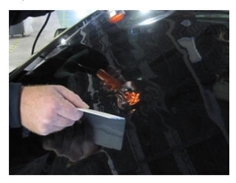
3. Once the tint is fully formed to the shape of the rear window, peel the backing away while soaking the tint with the shampoo/water solution as shown. Also soak the inside of the rear window at this point.
