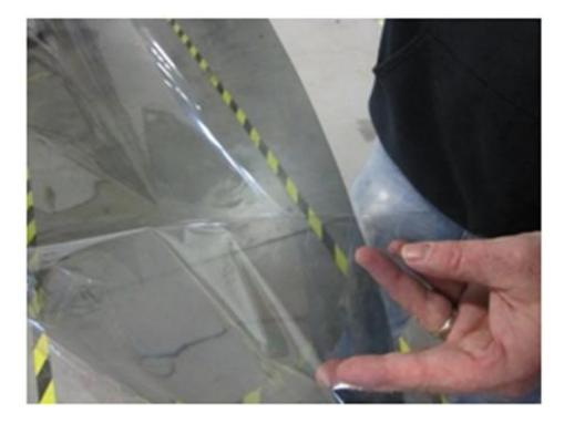
3. Soak the inside of the window in the shampoo/water solution and place the tint on the inside of the window. Position the tint so there is approximately 1/16" of glass showing at the top as shown below.
