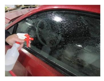
2. Peel the backing film from the tint and lay the tint on the outside of the window, adhesive side out. This is to have the tint in ready position when you are ready to position it in the inside of the window.
