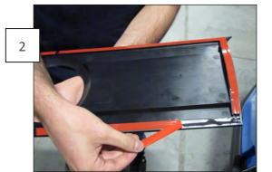
Peel the backing off the tape and line up the decklid panel on the trunk lid. \*\*\*It may help to test fit the decklid before peeling off the backing of the tape so you can see how everything is going to line up before the final installation.\*\*\*
