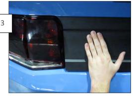
Once you have lined up the decklid panel, press firmly to set the adhesive tape.
