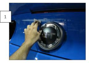
Using the supplied alcohol pad, wipe down the perimeter of the trunk lid where the tape will contact.
