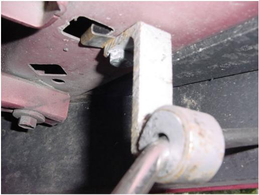
Below is an image of what not to do when completing this installation. Make sure that the U bolts holding the old 13. pipes onto the adapter are very tight. I did not tighten them down enough and the adapter slipped off of the passenger's side of the car. Unfortunately, the adapter kit would not fit back over the pipe so I needed to go to a local auto shop and purchase a coupling that would hold the adapter to the original pipe on the car.
