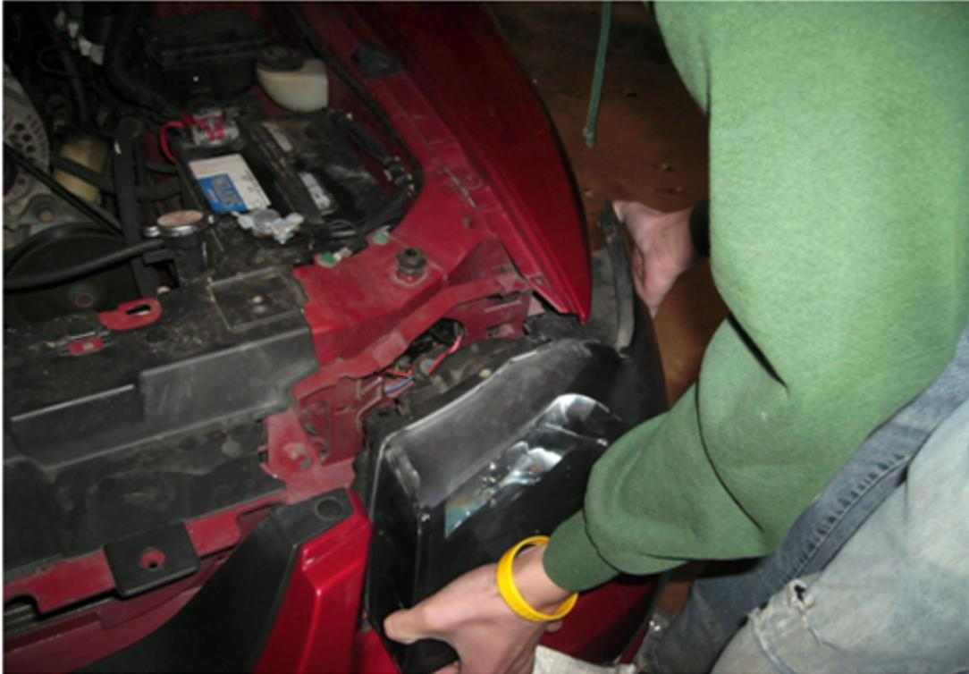
8. At this point, you will need to either disconnect the battery or remove the fuses for the headlights.
