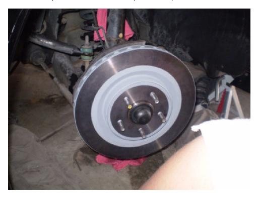
6. It is a good idea to use a little brake cleaner on the rotors before installing the new calipers. It is not required, but is good practice to insure everything is clean and won't damage the new pads. The new caliper can then be reinstalled using the same bolts and the same holes.
