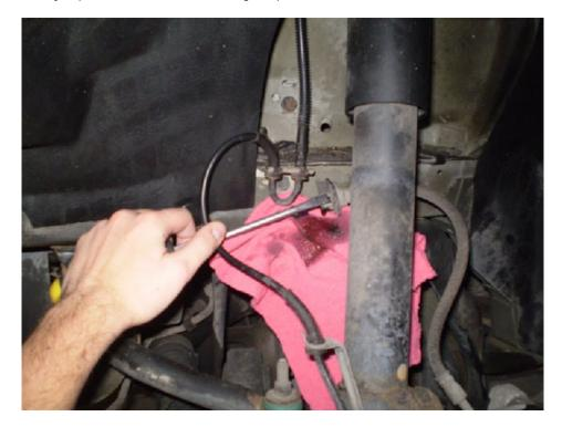
3. Then using a 15mm socket, the two bolts holding the caliper to the spindle can be loosen and removed. (Caution: the bolts holding the caliper may be rusted and hard to remove. WD-40 can be used to remove the rust and help the bolts to move. Let it soak for 10 minutes on bolts before trying.) After this the caliper should be free and can be removed from the car.
