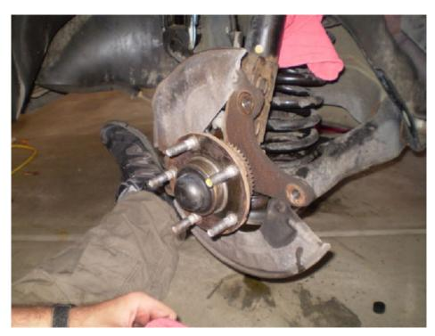
5. After cleaning, a small amount of anti-seize should be placed between the hub and rotor to make future removal easier. The new rotor can be placed back on the hub and the pushnuts be replaced.
