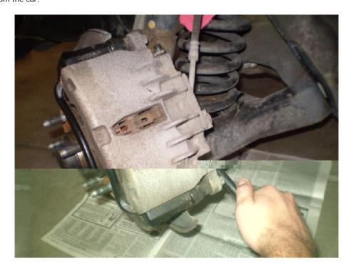
4. There may be some pushnuts holding the rotor to the hub, if so remove them and save them to replace back on the new rotor. Remove the rotor. (Caution: The rotor may be stuck to the hub and require a tap with a mallet to break it loose.) Once the rotor is removed, you should use a wire brush and a rag to clean the hub to help the new rotors seat properly.
