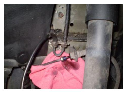
2. Using a flathead screwdriver, remove the retaining clip holding the softline to the body bracket. It is recommended that you place the end of the line as high as possible to reduce the amount of brake fluid that is spilled.
