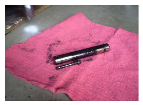
12. Once the differential pinion shaft is removed, the axle shaft can be pushed inward until rear axle shaft retaining uwashers at the button end of the axle shaft are clear of the side gear recess. From this position, the rear axle shaft retaining u-washers can be removed with a magnet. After this the axles can be pulled out of the housing and placed to the side.
