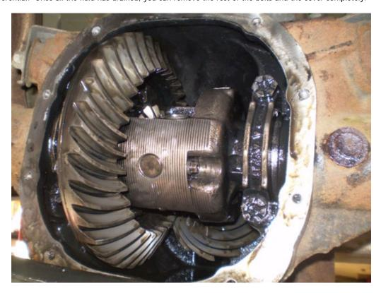
11. Once in the differential, you need to remove the differential pinion shaft bolt so that the differential pinion shaft can be puller out.
