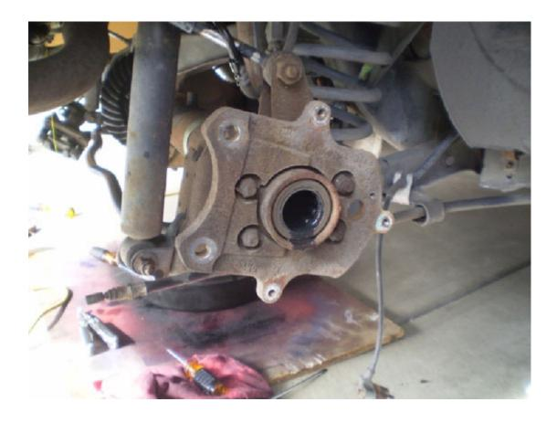
13. Once the axle is removed, the four bolts holding the caliper to axle bracket can be removed. Using the same bolts, the new bracket can placed back in the same spot. The new caliper brace can be installed using the new u-bolt and nuts and the new dust shield can be replaced.
