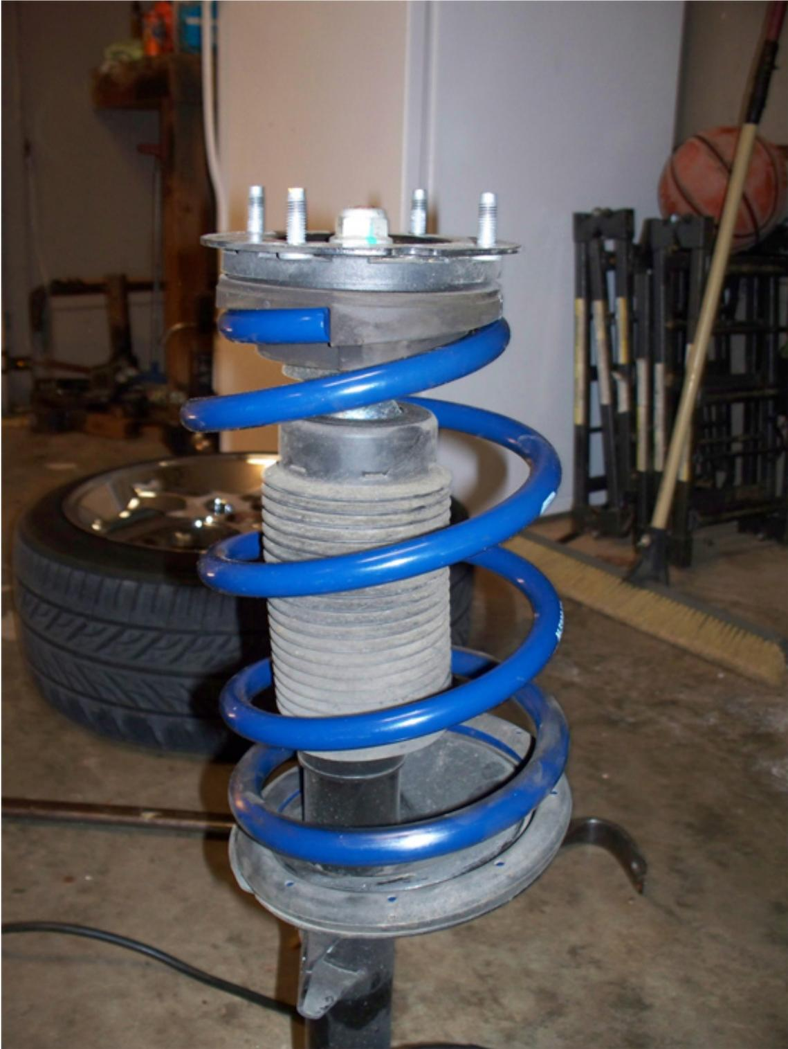
14. Place your strut assembly back into the strut tower bolting the top four bolts found in your engine bay first. Once this is done bolt everything back up and take it off the jack stands and move to the back of your car.
