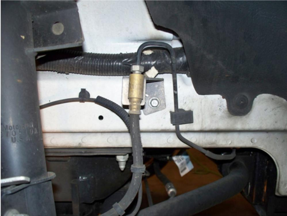
4. There is another 10mm bolt holding the brake line in place that is located behind the front strut the need to be removed also.
