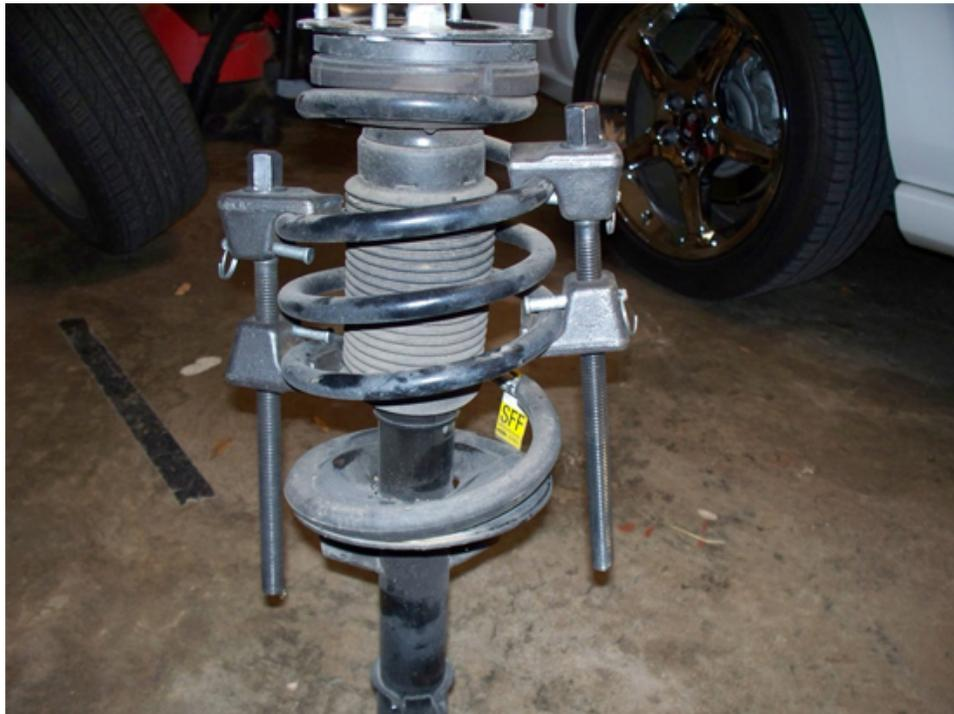
11. Now that the spring is compressed use a 22mm open end wrench to break the nut loose then you will need a 10mm open end wrench as shown in picture to remove the nut from the strut assembly. Once you have removed the nut pull the strut bearing cap off. (If the bearing cap does come apart don't worry it's not a big deal just place the bearings back into and put it back together.)
