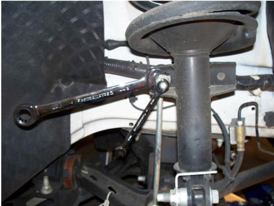
8. Now remove the two lower strut bolts and nuts from the spindle. (Use 18mm deep well socket with 6 inch extension.) Support the brake assembly with some wire or rope to lessen the strain on the brake lines on both sides.
