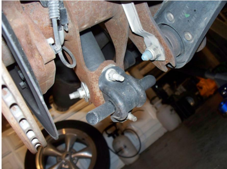
17. Remove the bolt holding your rear shock in place on both sides of your car. (Use 15mm deep well socket.)
