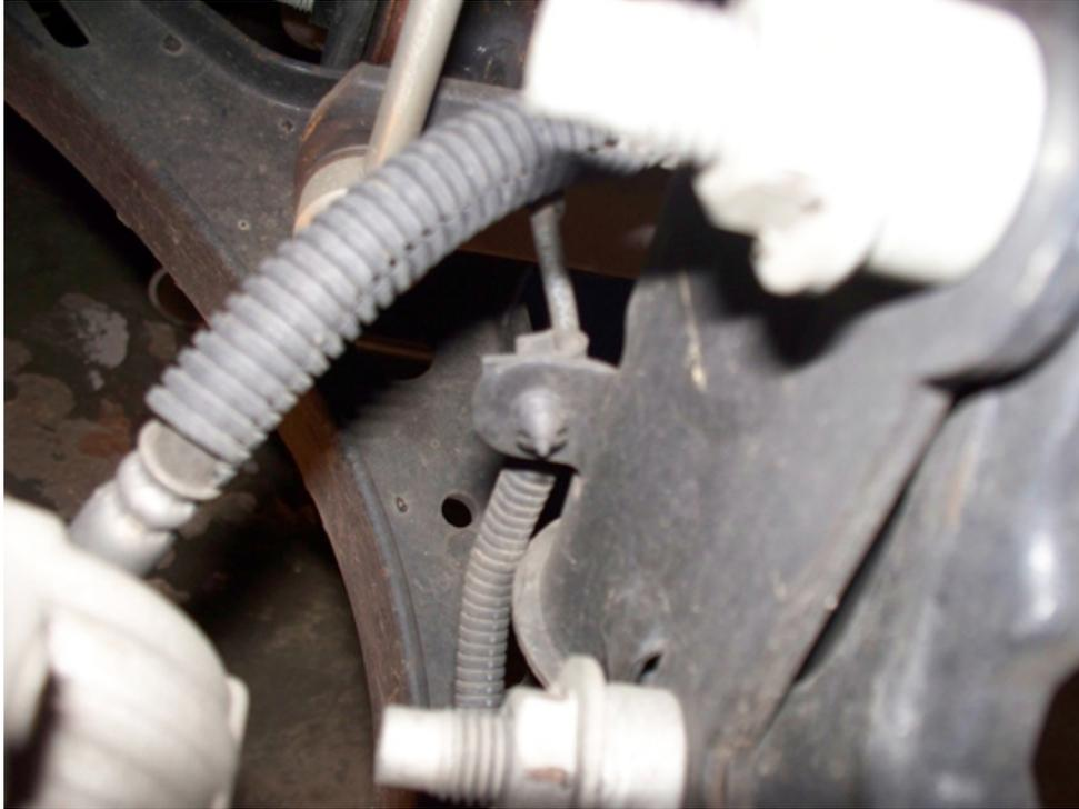
6. You will need to break lose the upper front anti-rollbar link from the strut housing. (Using 18mm deep well socket.)
