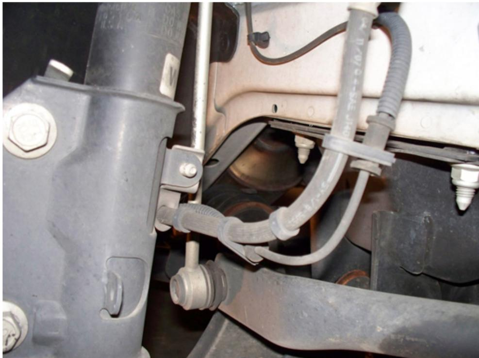
5. Now remove the ABS electrical wire support plastic one way clamp. (Needle nose pliers will help a lot when removing this.)
