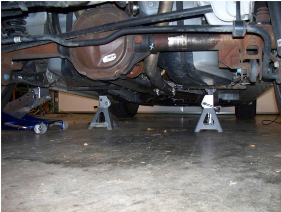
16. Unbolt your rear anti-rollbar clamps on both sides of your car and flip your rollbar to the rear of your car out of the way.
