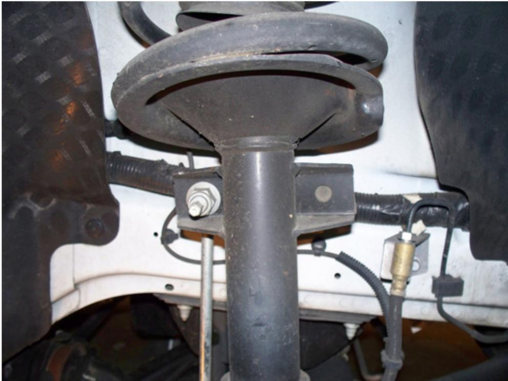
7. Once you have broke it lose you will now need to use an 18mm, 8mm Box End Wrench to remove the nut.
