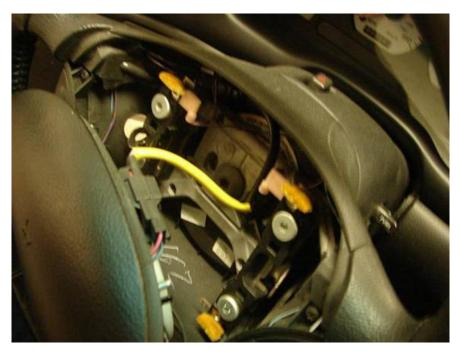
6. Carefully place the airbag in a safe place for now (we will re-install it on the new wheel). Make sure to put it face down (white plastic facing up)
