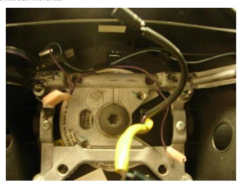
10. Now remove two Phillips head screws from each of the cruise control switches and set the switches aside for now (will re-install on the new wheel)
