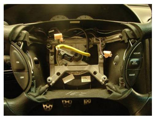
11. Remove the steering wheel bolt using the T50 Torx bit.
