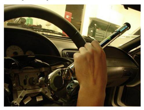
12. Now position the "gear/wheel puller" directly over the steering wheel shaft and slowly pull the wheel off the shaft using the puller. It shouldn't take a lot of force.
