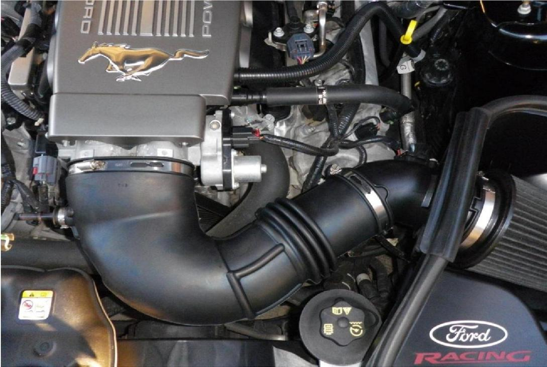
12. Reconnect the PCV line. Be careful not to damage the green retaining tab on the PCV fitting. The green retaining tab has to go over the ridge on the PCV tube.
