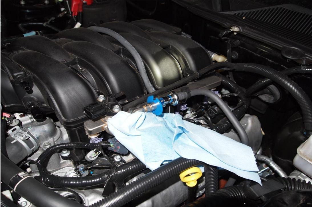
Remove the two bolts holding the fuel rails using an 8mm Deep Socket. After the bolts have been removed, remove the fuel rail with fuel injectors still connected
