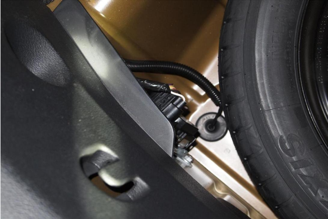
After the Module has been disconnected, start the car and run until it stalls and then crank the engine for an additional 10 seconds. Note, your car may or may not start.
