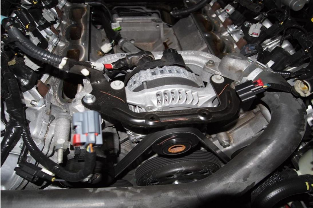
After Removing Bracket. Enlarge the bottom hole using 1/4" drill bit. After enlarging the hole, reattach the bracket and torque to 89lb per inch. You will need to bend the tab forward about 45 degrees to allow clearance for alternator wire.
