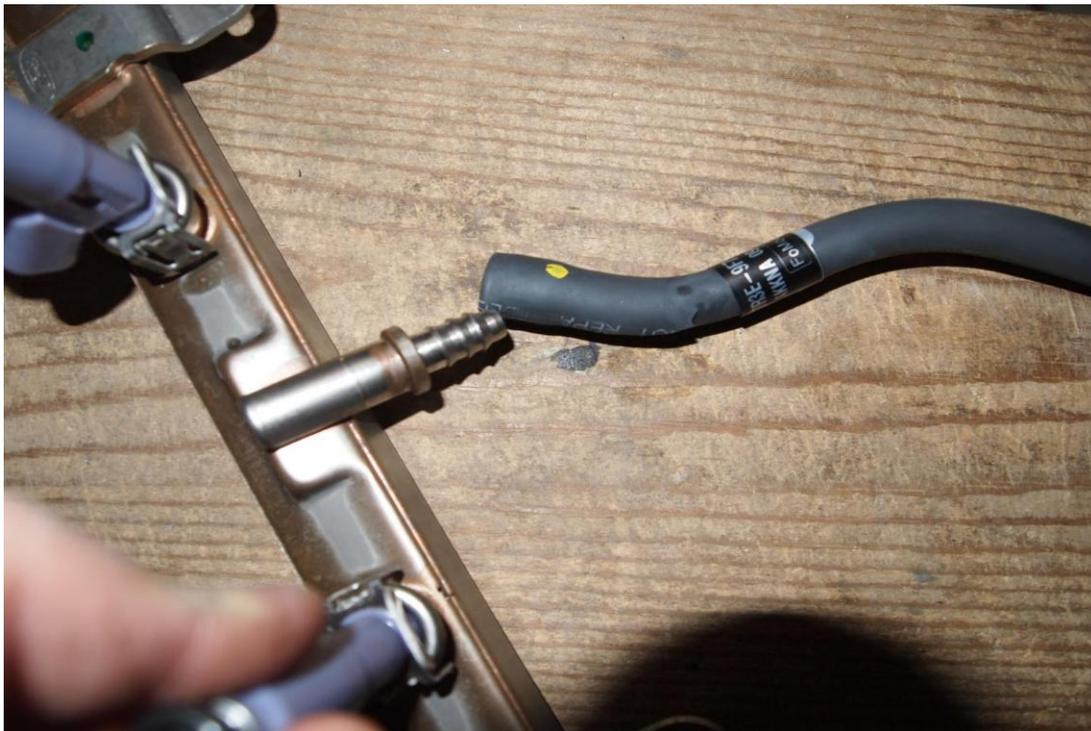
Reconnect fuel rails by pushing gently on fuel injectors to ensure they are seated. Attach new crossover line to fuel rail and used the supplied clamps. The clamps can be tightened with a flathead screwdriver
