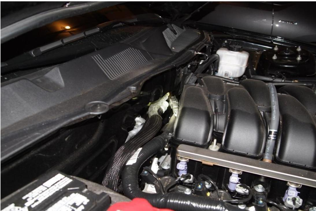
Step 3: (Disconnect Fuel Line and Remove [Fuel Rails](#))
