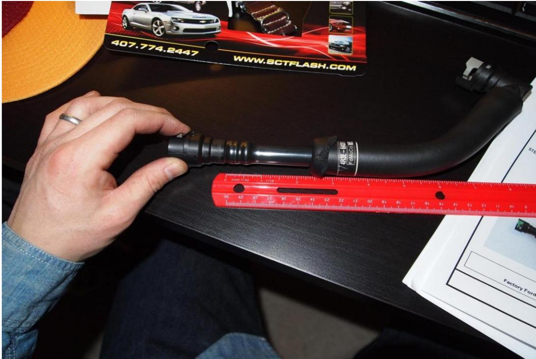
Measure 1.5" from the beginning of the tube but not from the connector and cut tube. Remove the connector and reattach by heating the end of the tube with a heat gun or hairdryer. The tube will shrink around the connector as it cools.
