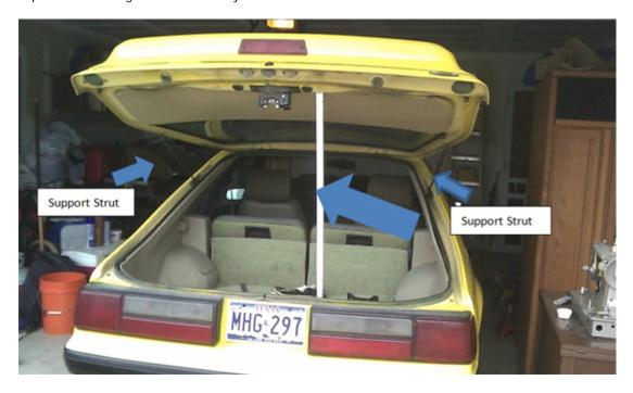
2. Now that the hatch is securely supported you can work freely underneath it. The supports are located on either side of the hatch held in place by a little medal clip. I found it easiest to work a little eyeglass flat head screw driver underneath one edge of the clip and to wiggle it around until it is about 2mm above the support strut. You should also start with the top of the support strut to make the bottom easier.
