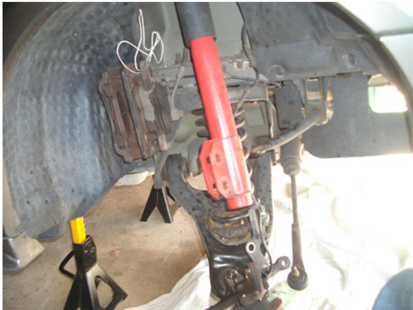
7. **Important:** Now SLOWLY lower the jack, making sure the spindle and control arm lowers as the jack is lowering. You will hear a loud POP! as the strut lowers, this is the sway bar coming off of the sway bar end. Make sure the jack and control arm lower **together!!** Now with all the components hanging down, use a prybar and pull the spring out (you might need to press down on the A-arm with your foot a bit, its ok).
