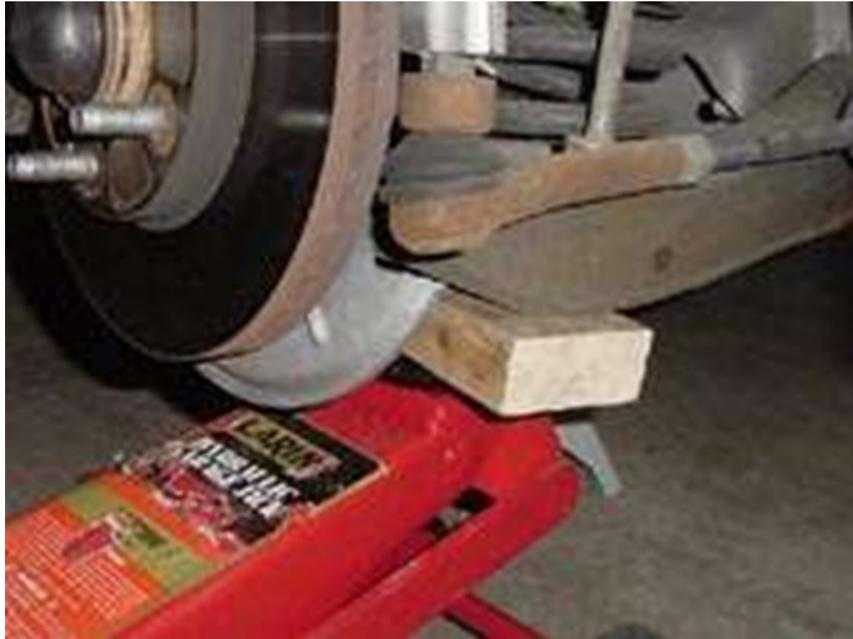
5. Now locate the tie-rod end. There will be a cotter pin which goes through a castle nut that secures the tie-rod end in place. Straighten the cotter pin out (it helps spraying this with WD-40) and pull it out of the castle nut. It takes some maneuvering but it will pull out. Remove the 19mm castle nut and then hit the top of the tie-rod end with a hammer. Give the top a few stern blows with a hammer and the tie-rod end will pop loose, let it hang down.
