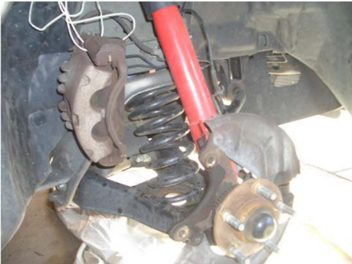
3. Next, remove the brake hoses from the small bracket behind the strut. Removing them from the bracket will give the hose some slack for when you disconnect the strut. You do not want to bend or twist these lines, so be careful, and let them hang down. You may be able to go on without this step if your very careful.
