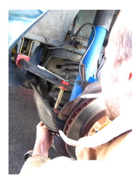
28. Reinstall the wheel and finger tighten the lugs. Release the jack from under the control arm and place it back under the frame rail. Jack up high enough to remove the jack stand then slowly lower the car.
