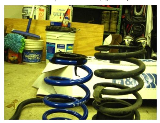
8. The lower pigtail on each rear spring needs to be pointing to the driverside of the car, make sure to do this correctly if not your rear end will sag lower then anticipated. The picture below illustrates its position.
