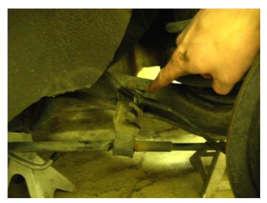
5. Place the small block of wood on the jacking cup and raise the jack so that it is contacting the rear of the control arm just under the bolt enough to take some tension off the bushing.
