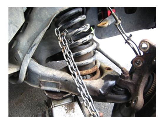
23. Slowly release the jack from under the control arm and allow the spring to expand, if necessary use the pry bar to pull out the spring the rest of the way, if there is any stored inertia from the spring the chain will retain it, unlock/unbolt the chain and remove the spring from the car.
