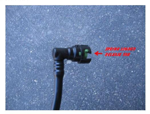
5. Remove the wiring harness from the MAF sensor. To do this, pull the red tab on the back and pull out the wiring harness from the MAF sensor. Remove the MAF sensor after you have assembled the new intake, so you do not lose it.
