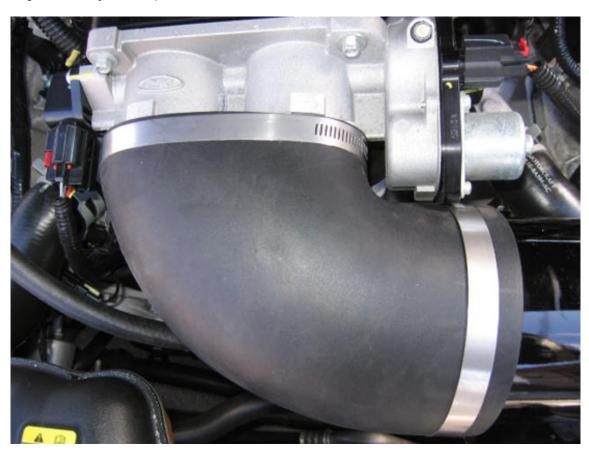
14. Once the elbow and clamp have been fitted on the throttle body, you may attach the PCV rubber tube to the valve cover, where it used to be attached.
