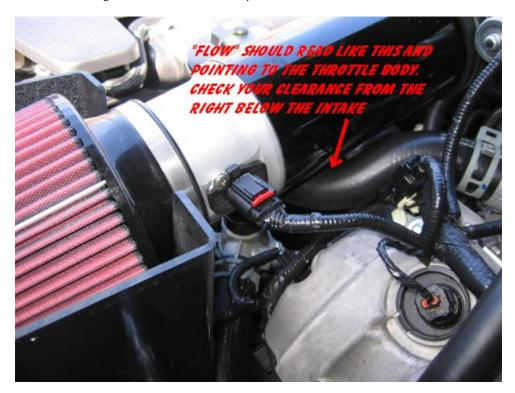
16. Once everything is together, adjust the intake so the filter is not touching the car and is only touching the shield. Tighten all 3 clamps, but do not over tighten them, they should just be snug.
