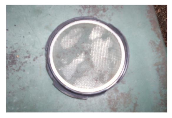
6. Adaptor attaches to MAF by using the 4 screws that are supplied, this adaptor is needed in order to use the air filter.
