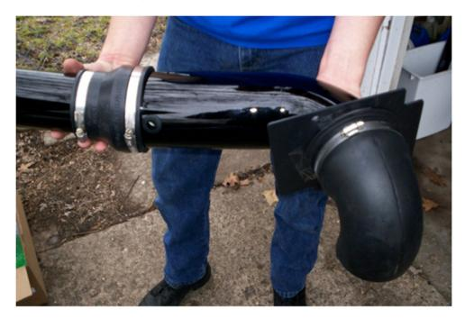
9. Install the MAF sensor; on the end of the 90 degree elbow make sure that the electrical plug is pointing towards the rear of the car. This position is necessary in order for the wires to reach the MAF sensor. Hose clamp will be placed over the elbow to secure the MAF to the pipe.
