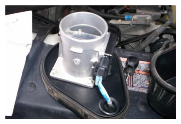
5. Remove MAF screen and install the supplied MAF adaptor. **Do not reuse the screen**.
