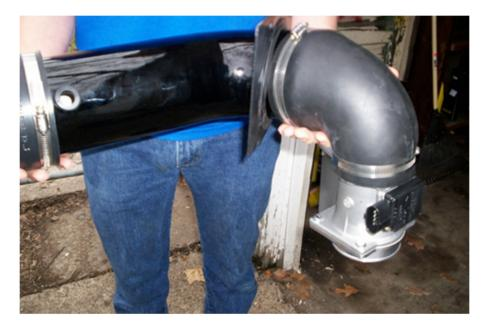
10. In order to install the JLT intake you must stand the pipe up and "screw" it into the hole in the apron. This is why the tape was placed earlier, use soapy water on the "U" channel gasket to prevent it from sticking to the tube.
