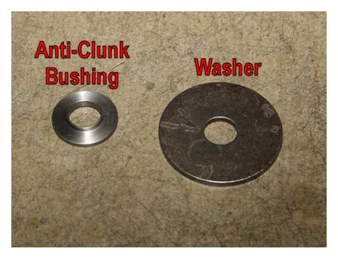
13. As shown below, use a washer between the control arm and the bracket. The anti-clunk bushing should be installed from the outer side of the bracket, and its smaller side will fit into the bracket's hole. Repeat this procedure for both the driver and passenger sides of the control arm. I will point out that it's a tight fit to get both washers in place, but with a little perseverance you'll get them installed and everything lined up.
