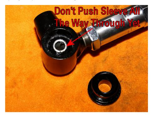
12. The J&M upper control arm makes use of a special anti-clunk bushing to help take up the slack between the bolt and the hole in the bracket. The difference in sizes can contribute to a clunking sound in the rear of the vehicle, even if the stock control arm is still installed. The anti-clunk bushing solves this issue. The standard washers are used to take up slack between the control arm and the bracket.
