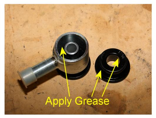
7. The assembled ends should look like the ones in the picture below. Don't forget to thread the jam nuts into place, and **keep in mind that one of the ends of the rod is reverse-threaded!**
