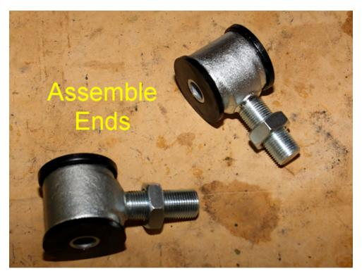
8. Thread the ends into the aluminum rod matching the amount of threads on each end, as you'll want the ends to be equal. Then place one of the bolts into both the factory bar end, and the J&M bar end, to hold them together.
