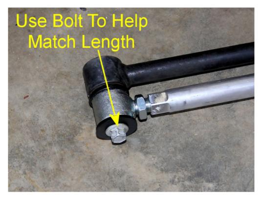
9. Turning both ends one turn at a time, to keep the amount they're threaded in matching, match the J&M panhard bar to the length of the factory bar. Use the other bolt to ensure the holes in the two bar assemblies are exactly equal. You'll perform your adjustment with the new panhard bar installed at the stock length. It's more difficult to install the bar, if the size is different than the factory bar which you removed.
