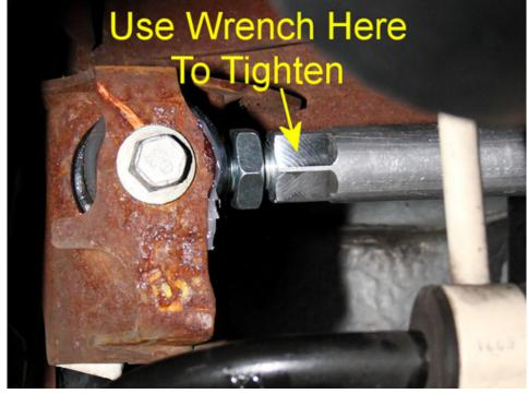
15. Finally, tighten down the jam nut on the other end of the panhard bar. This can be accomplished easily by spinning the nut with a 1-1/8 inch or adjustable wrench.
